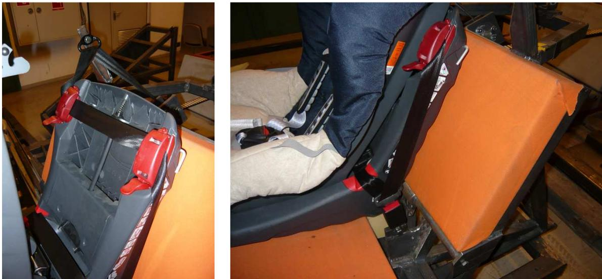
Figure 4: Installation with both belt clamps, view from driver's side
