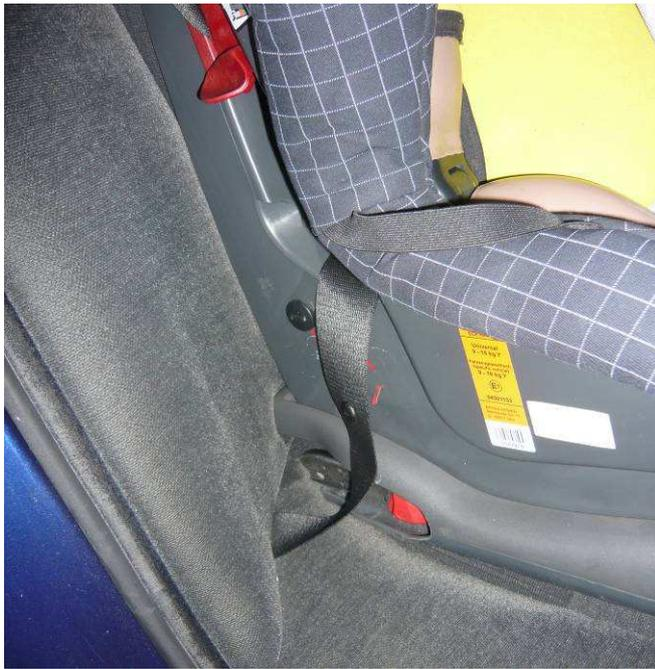
**Figure 1: Slack in vehicle belt**
