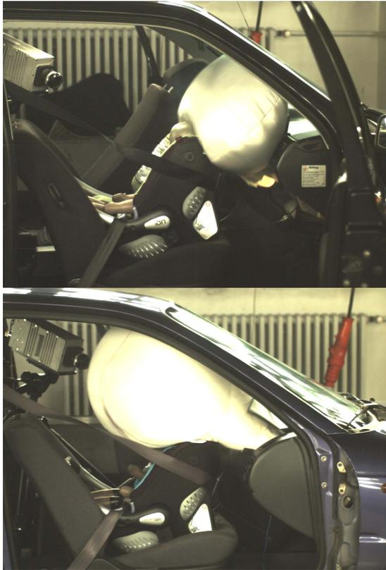
**Figure 4. Maximum airbag deployment: car 1 (top) and car 5 (bottom).**
