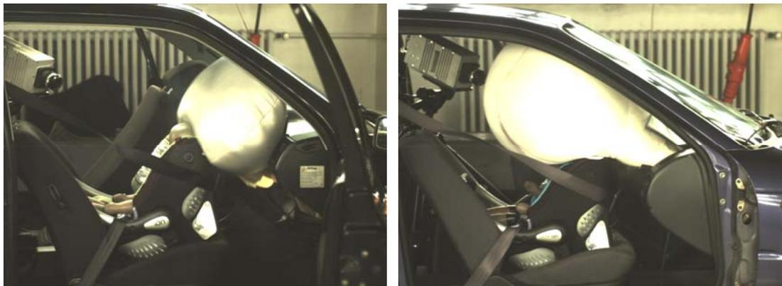
**Figure 5: Maximum airbag deployment: car 1, car 2**
