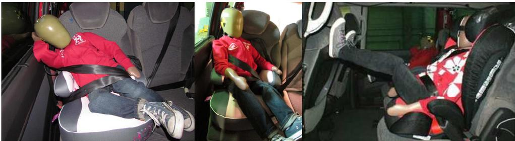
**Figure 5.2:** Posture position in combination with typical misuse – using a Q6 dummy
