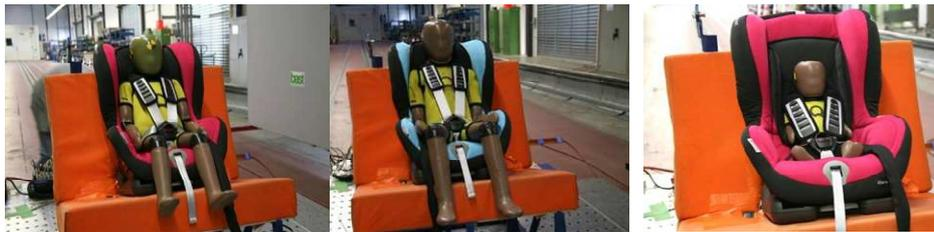
**Figure 4.2: Test set up with an ISOFIX CRS and Q3 (reference), Q6 (too heavy) and Q0 (too small)**
