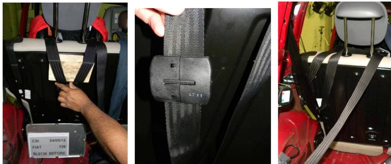
**Figure 3.3:** Illustrations of introducing slack in top tether, indicator not green and no top tether
