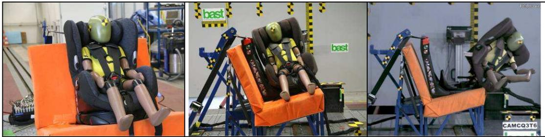
**Figure 2.2:** Configuration with seat shell turned 90°: Reference condition; misuse; during the test
