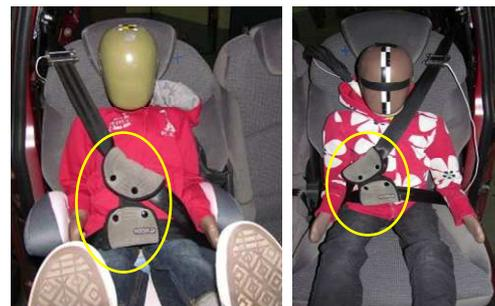
**Figure 1.4:** Seatbelt routes with “add-on” Q3 (on the left) and Q6 (on the right)
