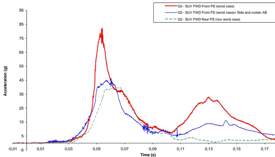
Figure 12: Head acceleration resultant of Q3 on the struck side
