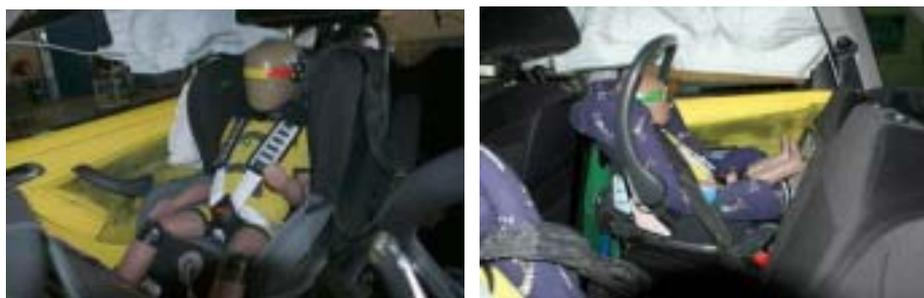
Figure 11 Final positions of dummies with inflated side airbags
