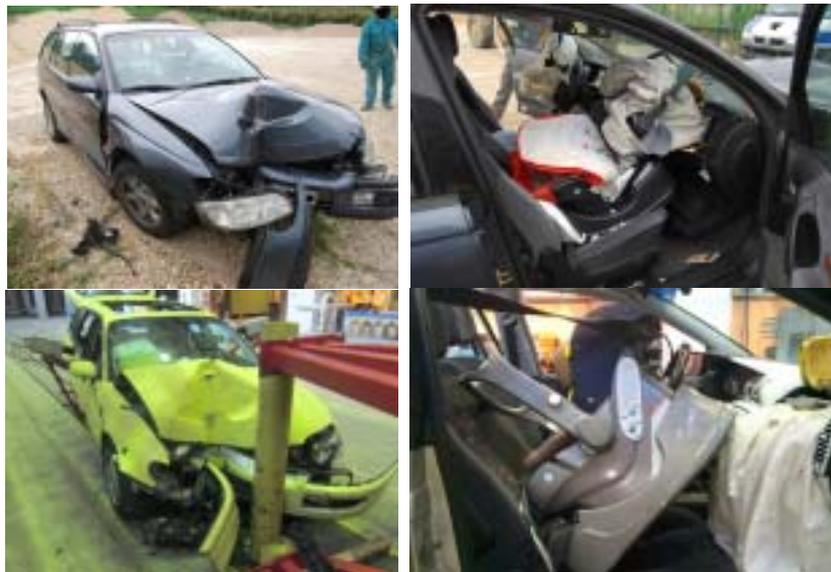
Figure 8: illustration of accident case and its reconstruction with frontal airbag deployment
