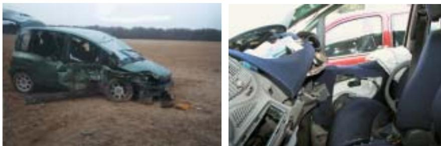
Figure 6: illustration of case n°1 with side airbag deployment
