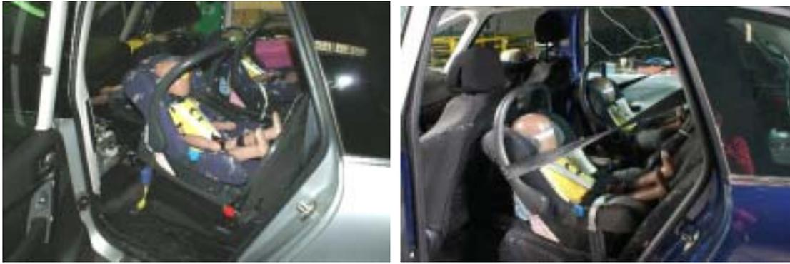
*Figure 15: View of the RWD FC CRS G0+ with and without the ISOFIX base*
