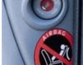
Figure 1: Key switch located on the extremity of the dashboard (right side)
